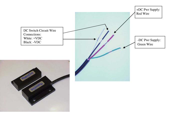
White Wire: +VDC on Switched DC circuit
